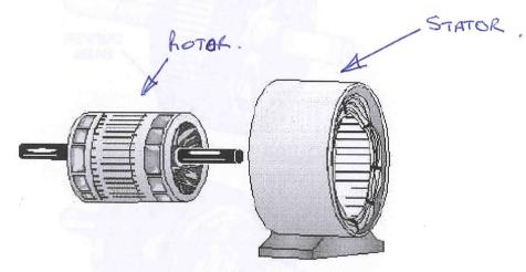
For higher-power applications where a polyphase electrical supply is available, the three phase (or polyphase) AC induction motor is used. The phase differences between the three phases of the polyphase electrical supply create a rotating electromagnetic field in the motor.
