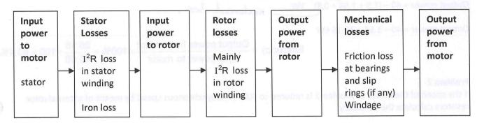
$$Efficiency = \frac{Output power from motor}{Input power to motor} \times 100\%$$
